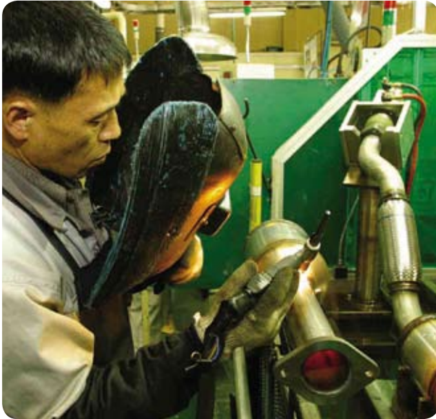
Exhaust system welding, grade 439, S. Korea.
